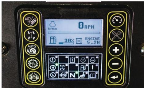
**KNOWLEDGE ON DISPLAY.** An integrated display allows the operator to optimize machine performance by adjusting operating attachment and ground drive parameters while providing machine diagnostic information including: engine rpm, fuel level, battery voltage, engine coolant temperature and engine hours.
