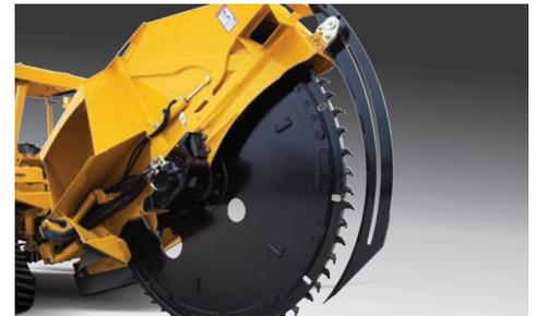
**AN ATTACHMENT FOR EVERY JOB.** The RTX1250 has an arsenal of attachments to match many applications including rockwheels, plows, combos and trenchers.
