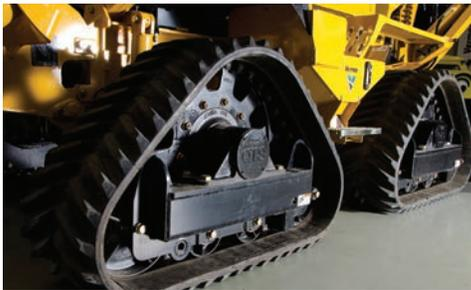
**QUAD TRACK ADVANTAGE.** The optional quad track system offers reduced surface damage and increased tractive effort
