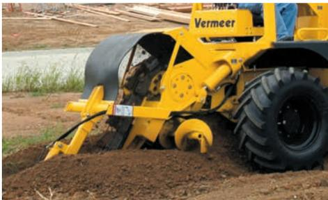
**MAKE SENSE OF YOUR TRENCH.** When difficult ground conditions are encountered while trenching, causing a sudden drop in engine speed, the TrenchSense™ feature automatically pauses the forward motion of the tractor to prevent engine shutdown and recalibration of the machine controls. Once preset engine and trencher speed recovers, forward AutoCreep resumes. The sequence occurs within seconds and requires no operator adjustment.
