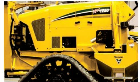
**INCREASED POWER.** When the RTX1250 engine drops from 2500 rpm to 3000 rpm under load, the horsepower increases from 120 hp (89 kW) to 125 hp (93 kW) allowing the RTX1250 to run at maximum horsepower in work mode.
